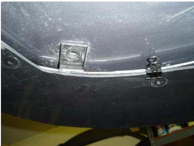
Photo 1-C: Clip holding the Air Splitter near the end
