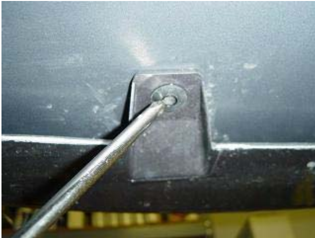
Photo 1-A: Release mounting clip on air dam
