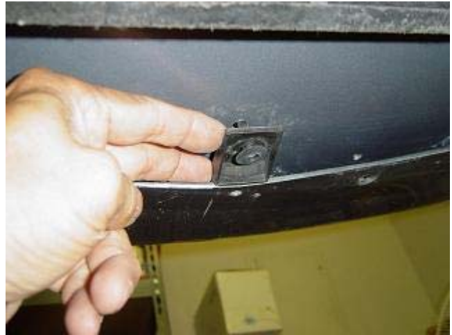
Photo 1-B: Pull air dam down to release clip
