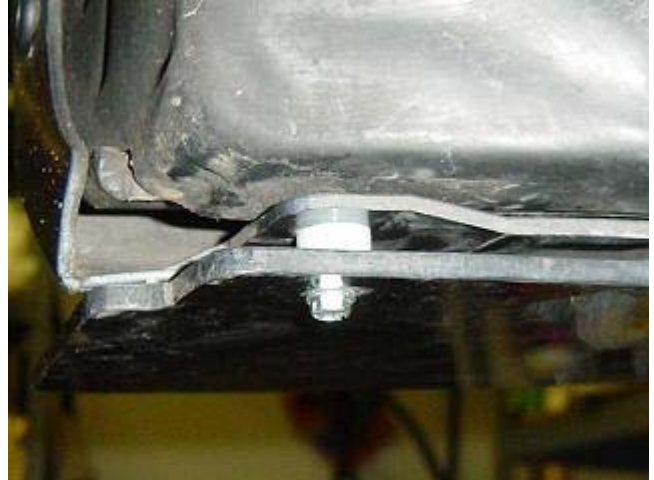
Photo 1-F: Air Splitter attached to the factory mounting hole
