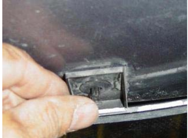
Photo 1-K: Air dam clip reattached
