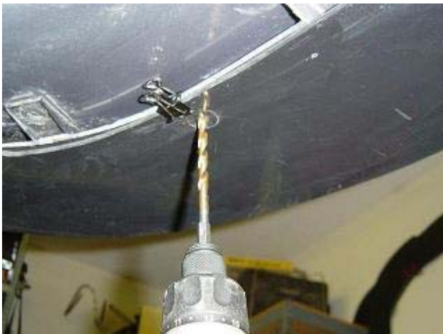
Photo 1-G: Drill using hole as a guide
