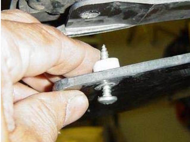
Photo 1-E: Supplied screw and spacer
