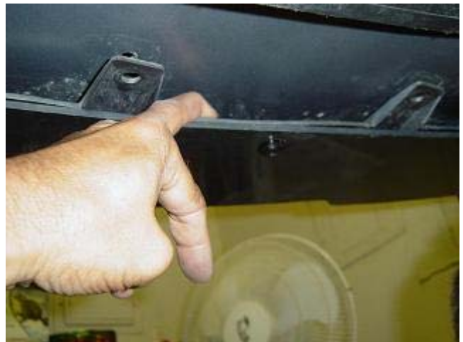
Photo 1-H: Pull air dam down for better access
