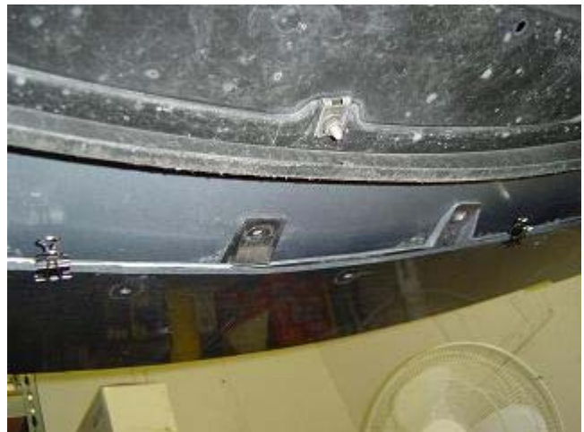
Photo 1-D: Clip holding the Air Splitter in the middle
