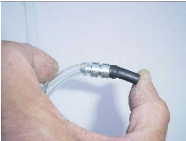
Photo 1: Remove the end piece from the hose
