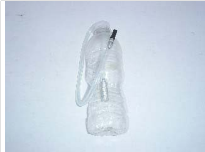
Photo 5: Install hose assemble into plastic bottle
