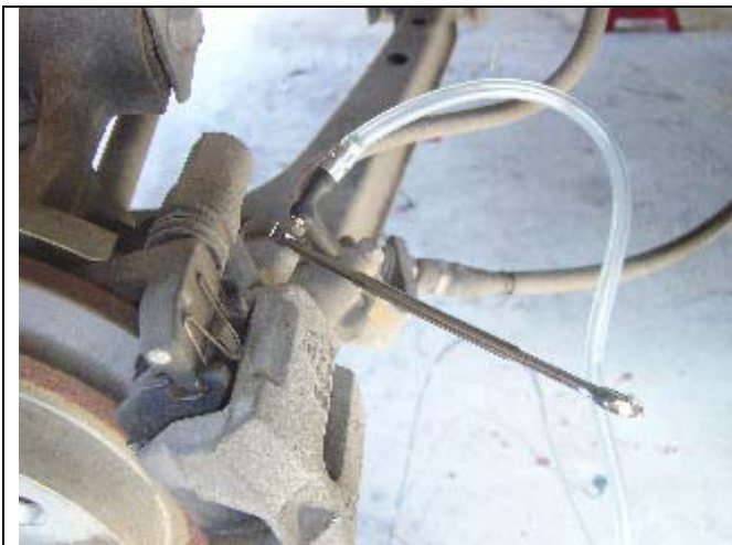
Photo 7: Attach wrench and bleeder hose
