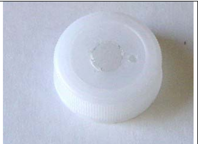
Photo 2: Drill holes in cap
