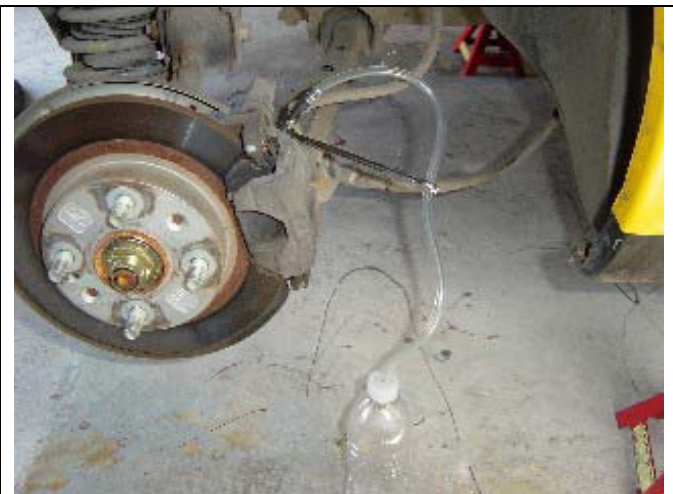
Photo 8: Make sure bottle is secure while bleeding
