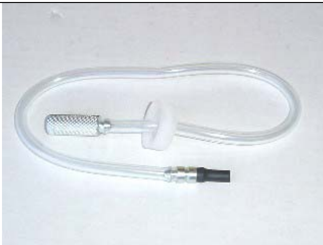
Photo 3: Install hose in to the cap
