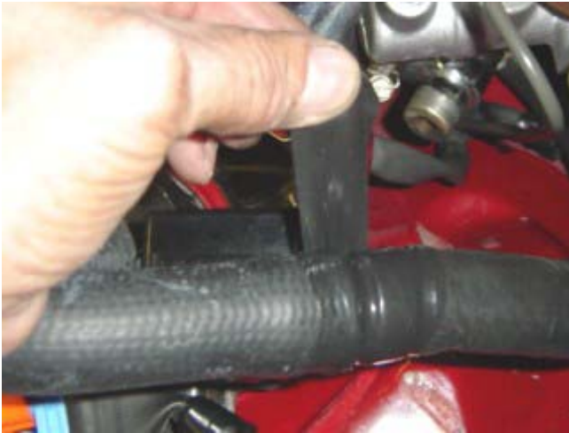
Photo C: Put silicone tape over hose connection
