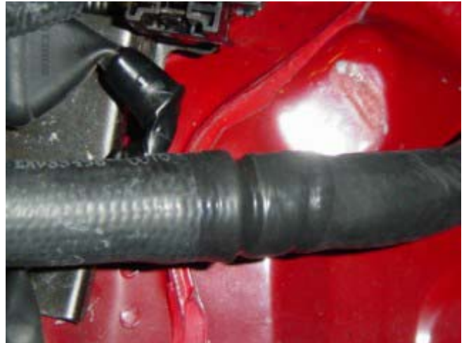
Photo D: Silicone tape complete
