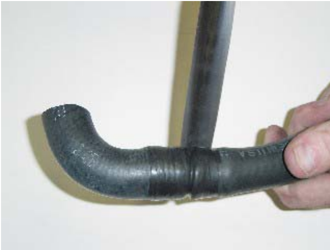
Photo G: Apply silicone tape around fitting
