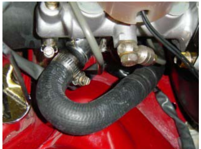
Photo F: Attach bypass hose using existing clamp
