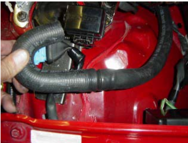
Photo E: Cut 3/4" off the intake fitting side
